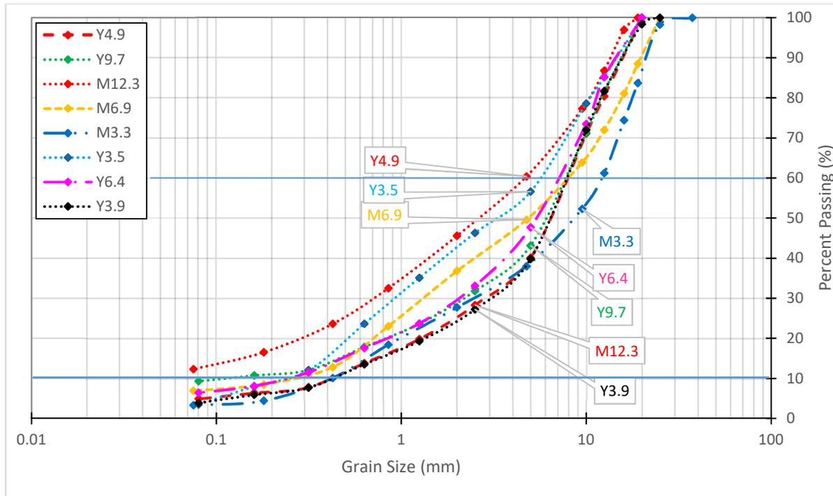
Figure 3 Aggregate gradation
