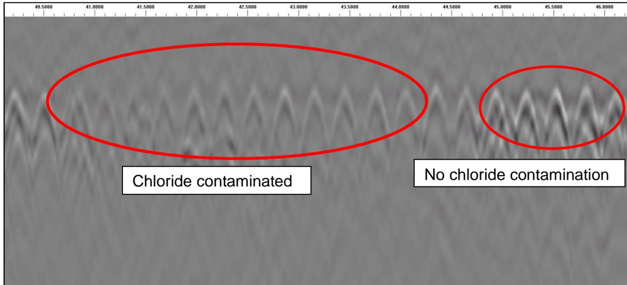
**Figure 2: Sample of Potential Deteriorated Rebar**
