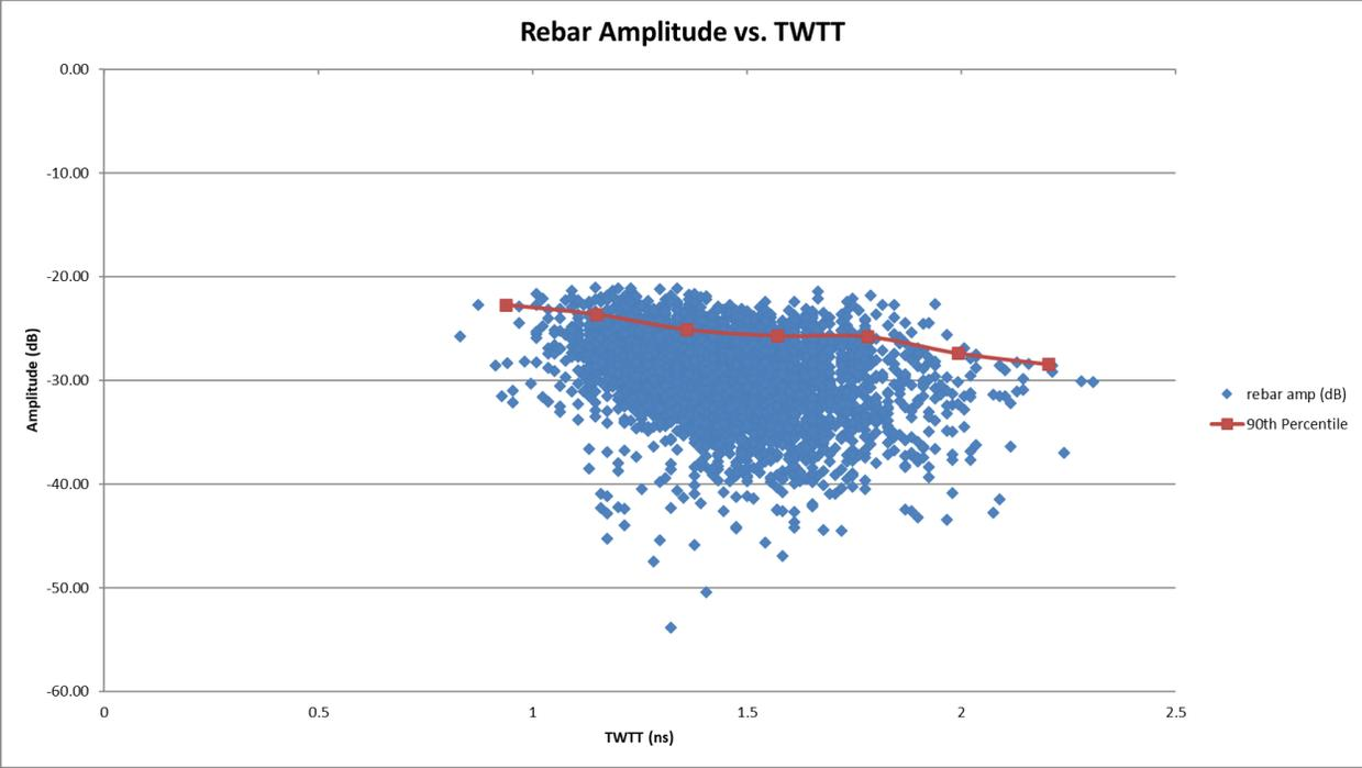
Figure 11: Rebar Amplitude and 90<sup>th</sup> Percentile Curve
