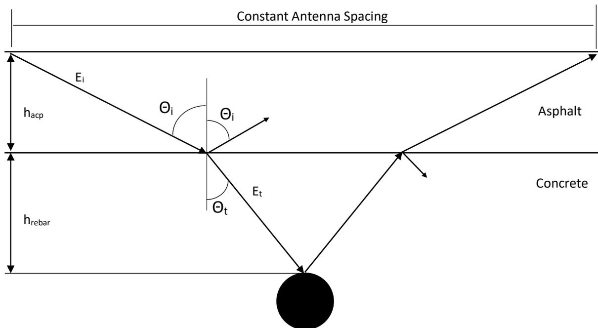
**Figure 9: Wave Path with Reflection and Transmission Angles Noted**
