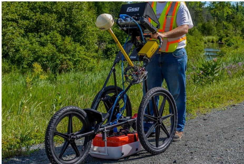
**Photo 1: GPR Unit Used for Data Collection**
