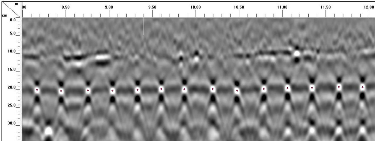
Figure 4: Sample of Rebar Selection
