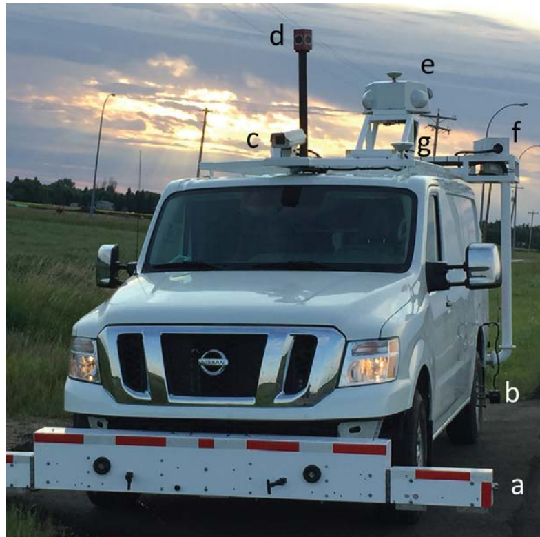
Figure 1 Pavement Surface profiler platform comprises of (a) Inertial Laser Profiler (b) Distance Measurement Instrument (c) Right of the Way Camera (d) Panoramic Camera (e) two LiDAR 360° Sensors (f) Laser Crack Measurement System (g) Inertial Movement Unit and GPS.
