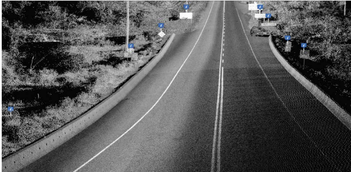
Figure 3. LiDAR pointcloud data collected at highway speed displaying its optical intensity. Notice that the traffic signs are marked automatically using machine learning algorithm.
