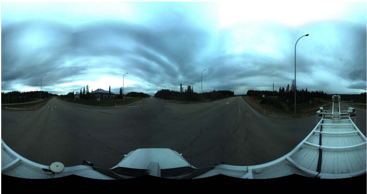
Figure 2, High resolution panoramic image collected from Tetra Tech PSP-7000 mobile mapping at highway speed. This panoramic image gives the user unique access to look around at all directions even at very low-light.
