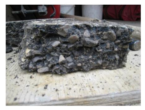
Photograph 1: Asphalt stripping visible in a piece of the asphalt mat obtained from the runway pavement.
