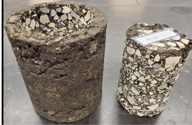
**Figure 12 Gyratory compacted sample for flow number test after surface cut and core**
