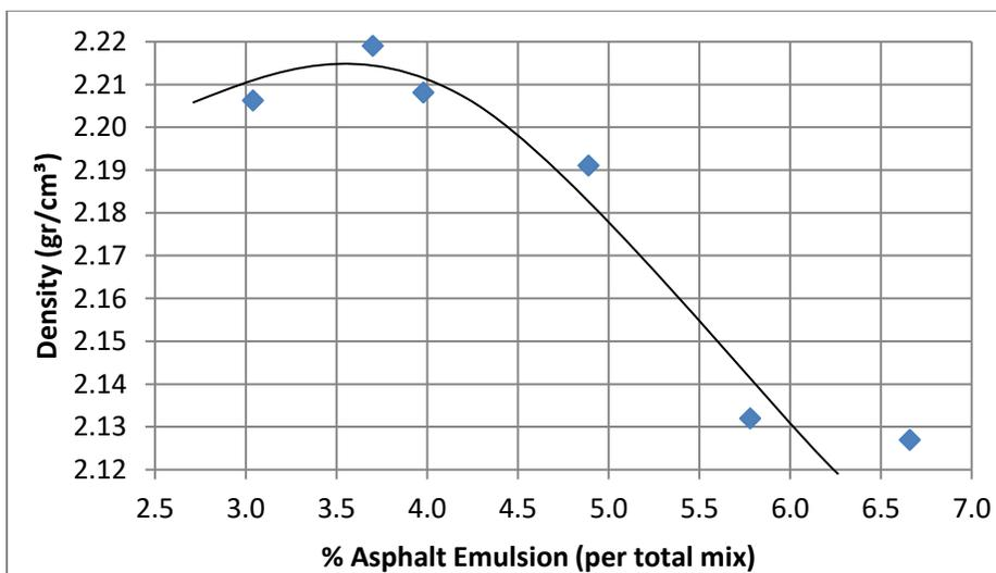
**Figure 5 Density vs. Asphalt emulsion content**
