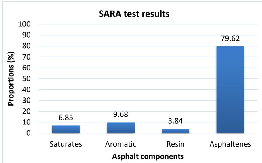
Figure 3 Asphalt binder components using SARA test
