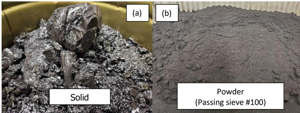
**Figure 2 Asphaltenes provided for mixing solid form (a), powder (b)**
