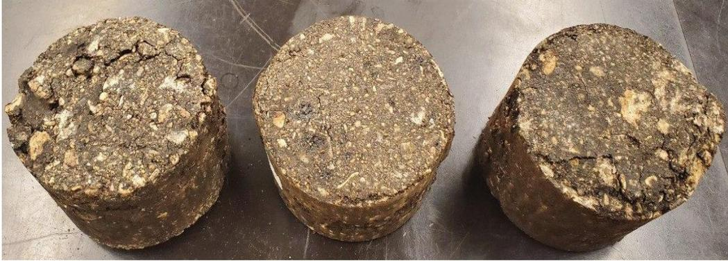
**Figure 8 Samples after performing Marshall stability test**
