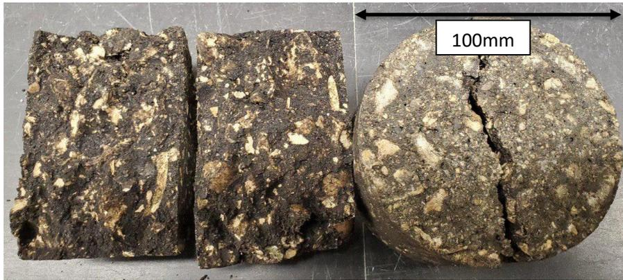
**Figure 7 Compacted samples by Marshall hammer after performing ITS test**
