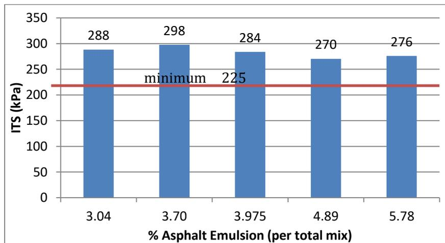
Figure 6 ITS results for mix design samples
