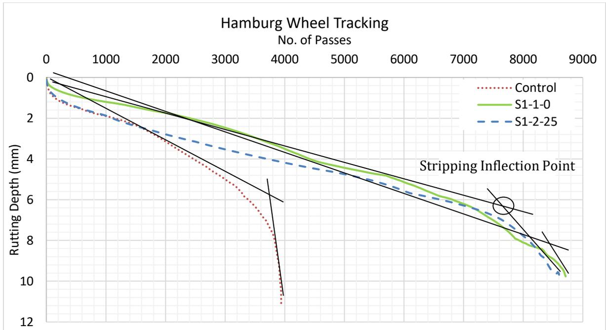
Figure 9 Hamburg wheel tracking results
