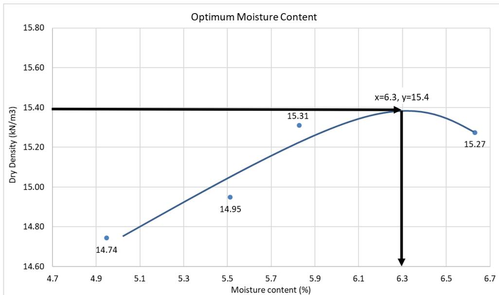
**Figure 1 Proctor test results**
