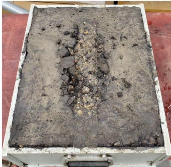
Figure 10 Slab sample after HWT test
