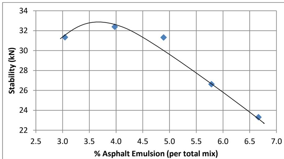
**Figure 4 Stability vs. Asphalt emulsion content**
