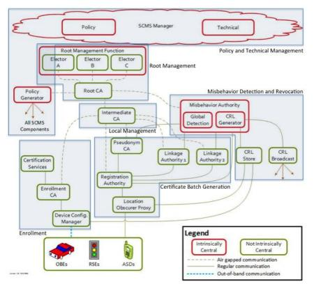
Figure 1. Annotated SCMS Architecture Diagram.
