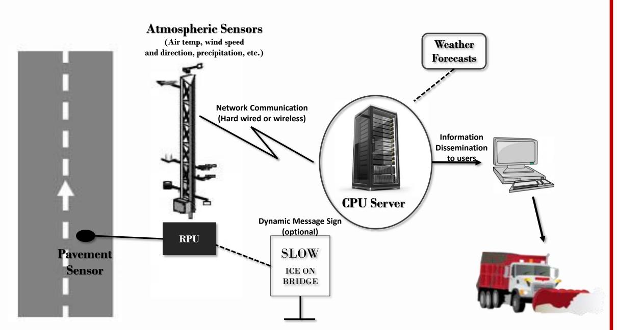
Road weather information systems (RWIS) provide information on current and near-future road weather conditions based on the data gathered at **RWIS** stations.
