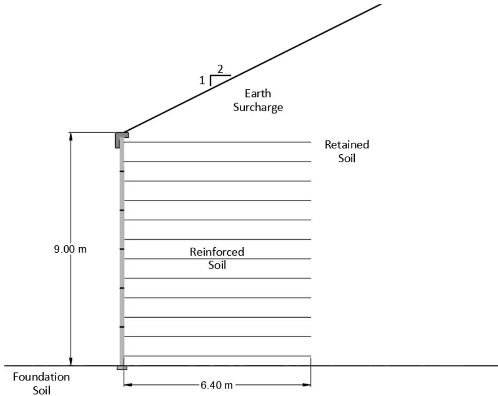
**Figure 4. Typical 2:1 wall section.**
