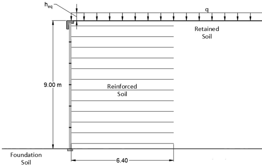
**Figure 3. Typical Flat-Top Wall Section.**
