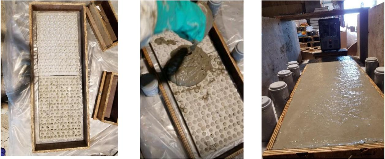
Figure 1 – Restrained plastic shrinkage
