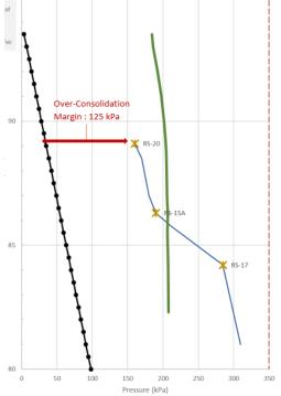
Figure 4 Effective and Pre-Consolidation Pressures Vs Elevation \_ Baseline Data
