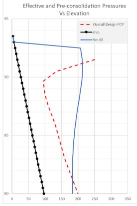
Figure 7 Additional loading as a result of embankment construction
