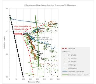
Figure 5 Effective and Pre-Consolidation Pressures Vs Elevation \_ Supplementary Data
