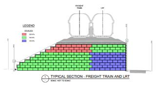
Figure 15 EPS Embankment configuration
