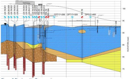
Figure 3 Stratigraphic Cross-section
