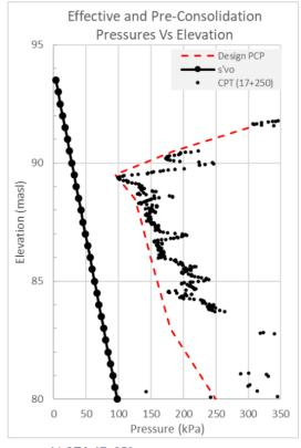
b) STA 17+250 Figure 6 Optimized Effective and PCP Vs Elevation
