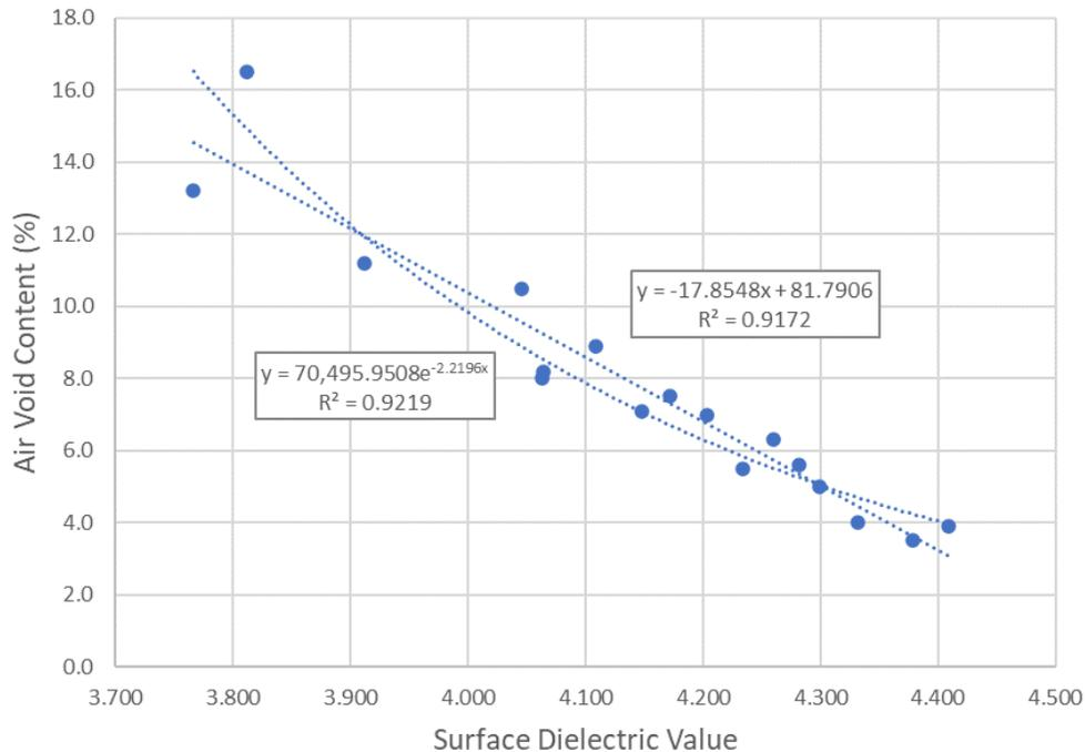
**Figure 3 – Relationship between surface dielectric value and air void content.**
