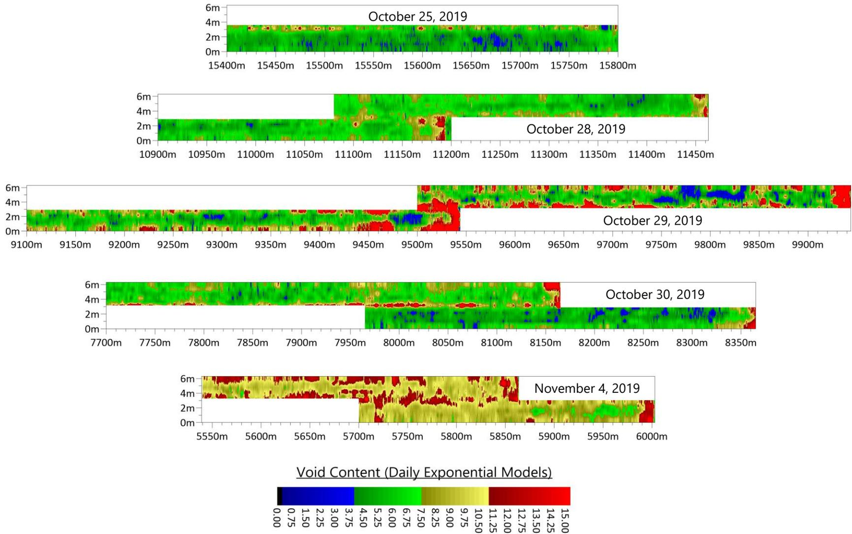
**Figure 6 - Variation in interpreted void content over test sections.**
