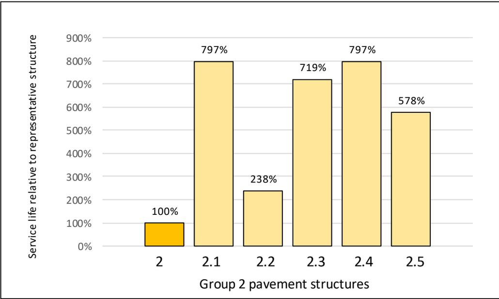
Figure 13. Comparison of predicted service life of group 2 pavements relative to structure 2.
