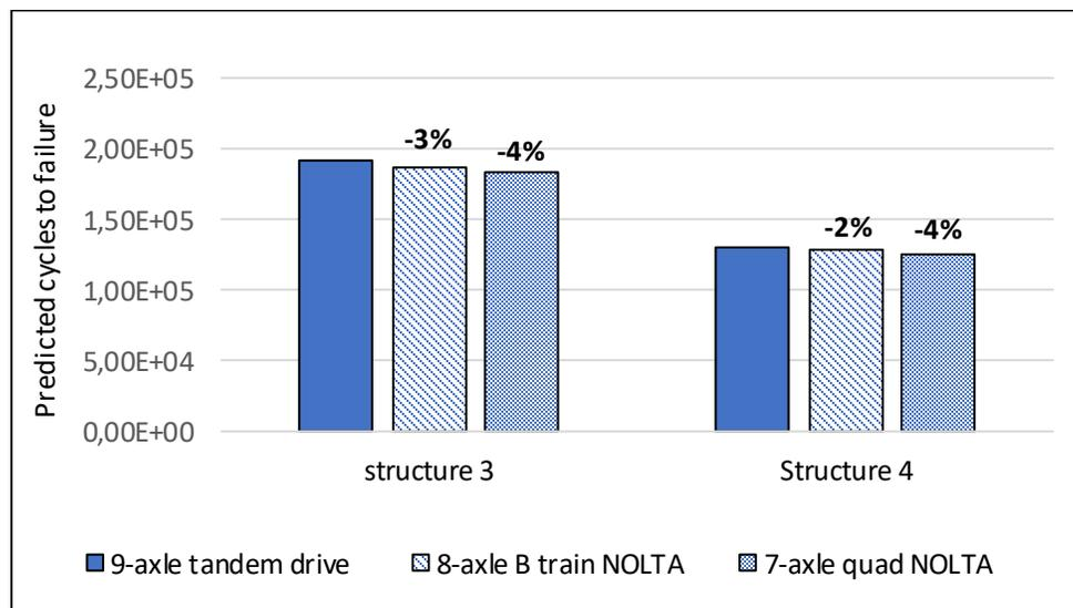
Figure 11. Long-term damage results for structures 3 and 4.
