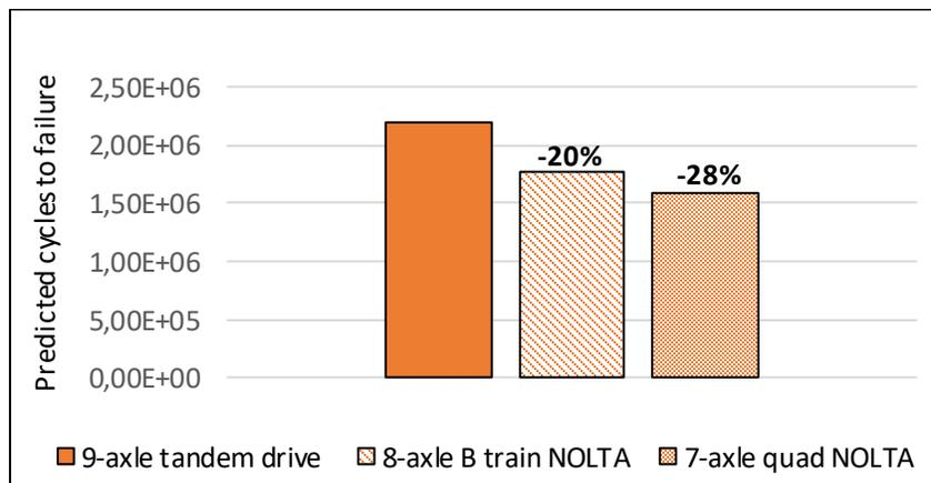
Figure 9. Long-term damage predictions for structure 1.
