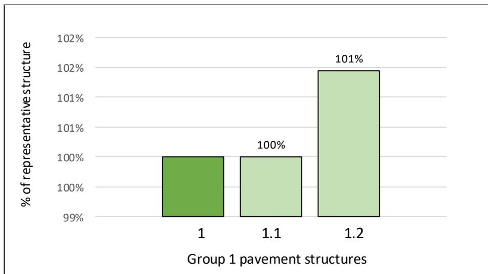
Figure 12. Comparison of predicted service life of group 1 pavements relative to structure 1.
