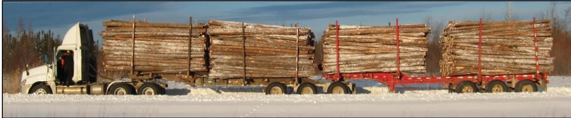
Figure 1. Example of tandem-drive 9 axle B-train.
