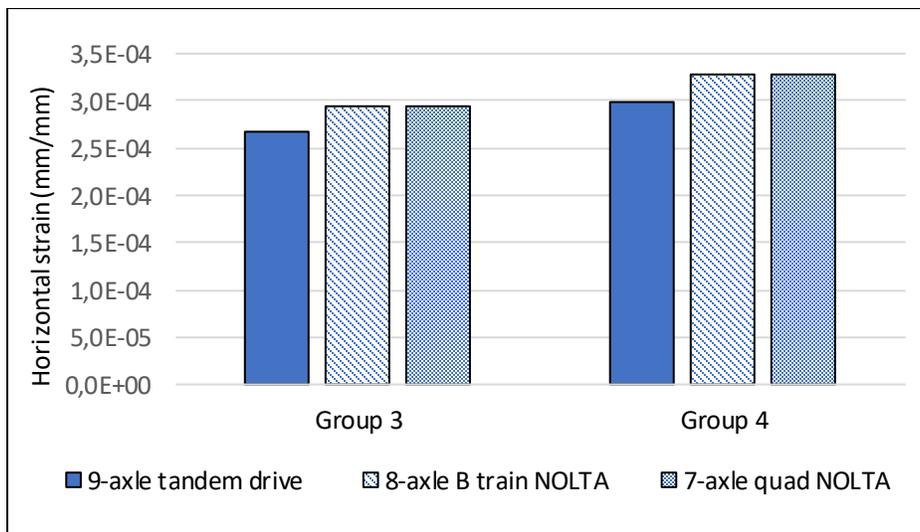
Figure 7. Comparison of HMA horizontal strains from 3 truck steering axle loadings.
