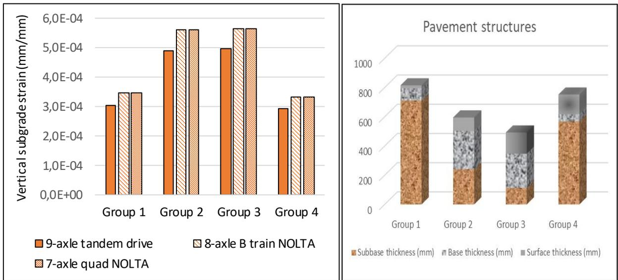
Figure 8. Comparison of vertical subgrade strains in four representative pavements (left) and graphic illustration of the representative pavement structures (right).
