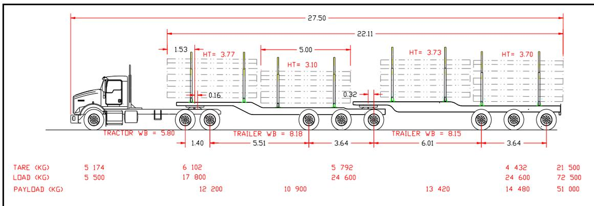
Figure 2. Proposed 72.5-tonne tandem-drive 9-axle configuration (dimensions in meters).
