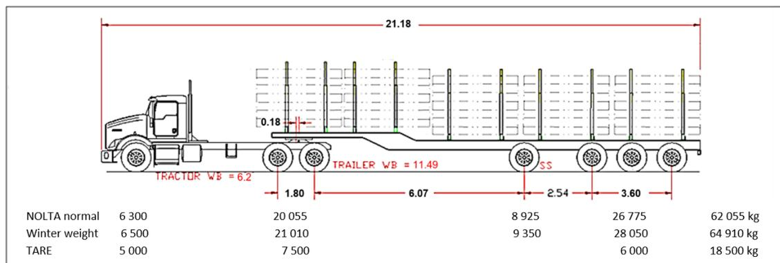
Figure 4. Reference vehicle: 7-axle tractor/4-axle semi-trailer.
