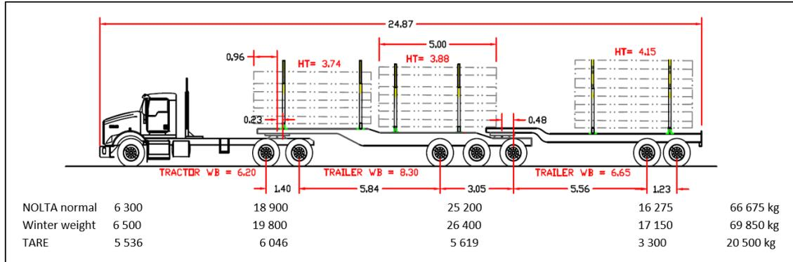
Figure 3. Reference vehicle: 8-axle log B-train.
