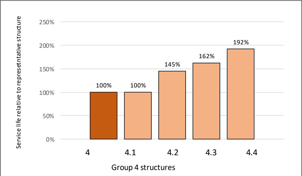
Figure 14. Comparison of predicted service life of additional group 4 pavements relative to structure 4.
