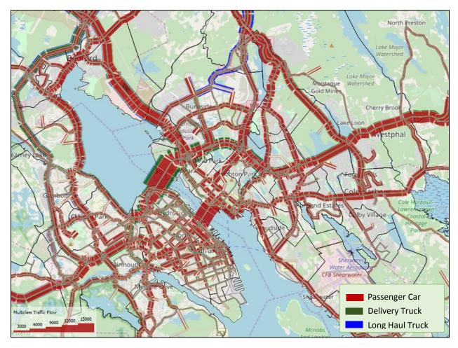
FIGURE 5 Result of multiclass traffic assignment
