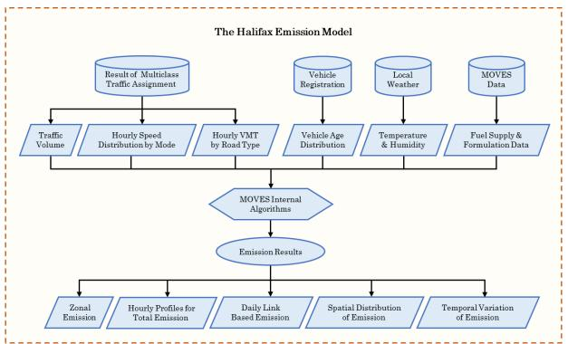
Figure 3 Framework for Emission Estimation from Multiclass Traffic Assignment
