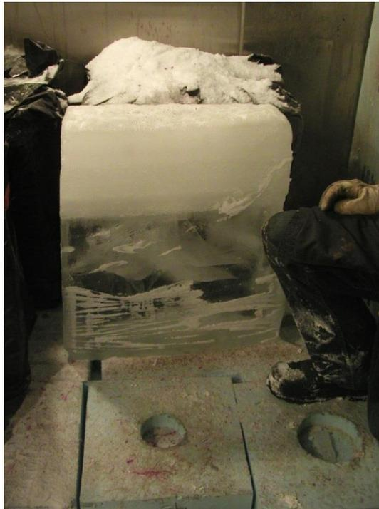
Figure 4: A block of ice showing clear ice (bottom of the ice block) and white ice (top of the ice block), the latter with internal layering.
