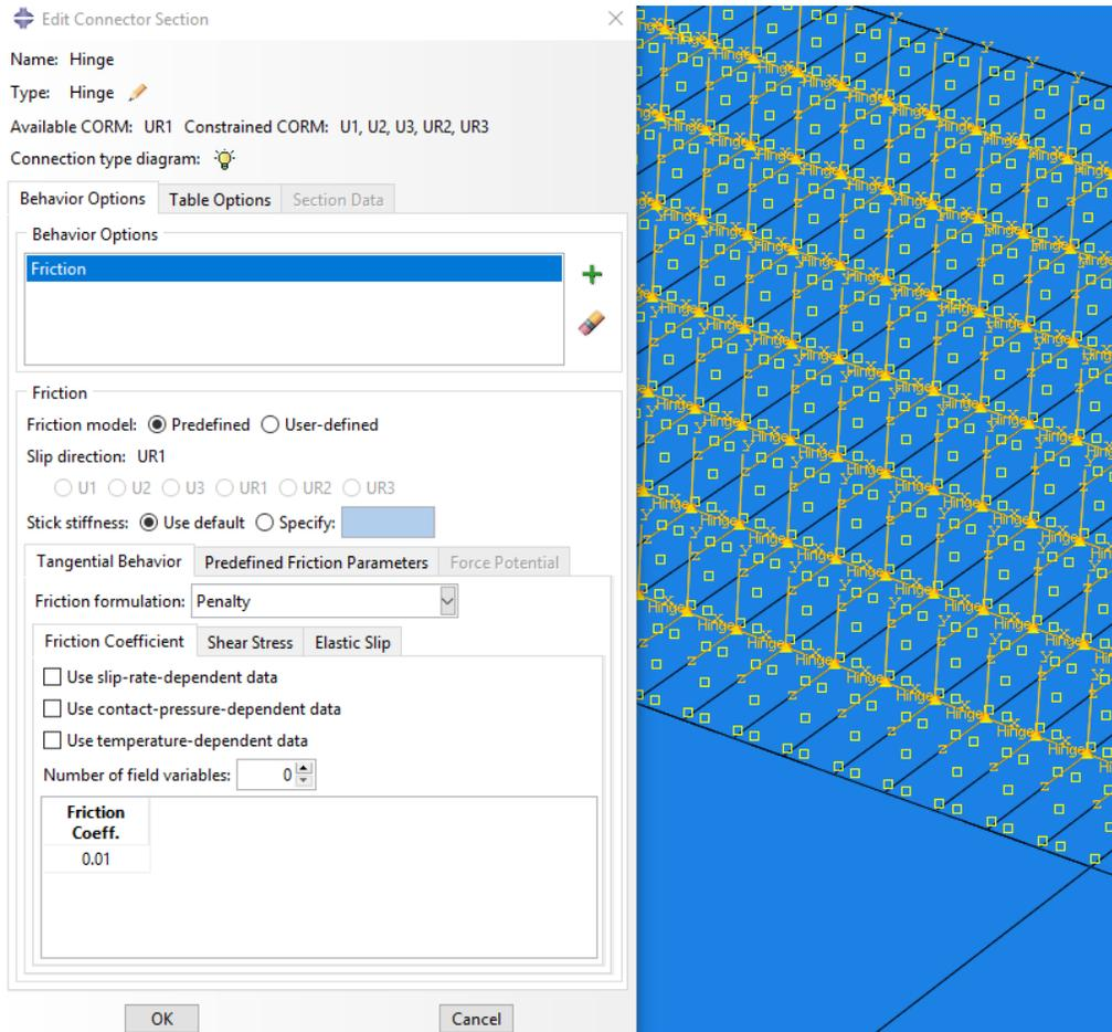
Figure 7: Definition of the hinge connectors in ABAQUS.
