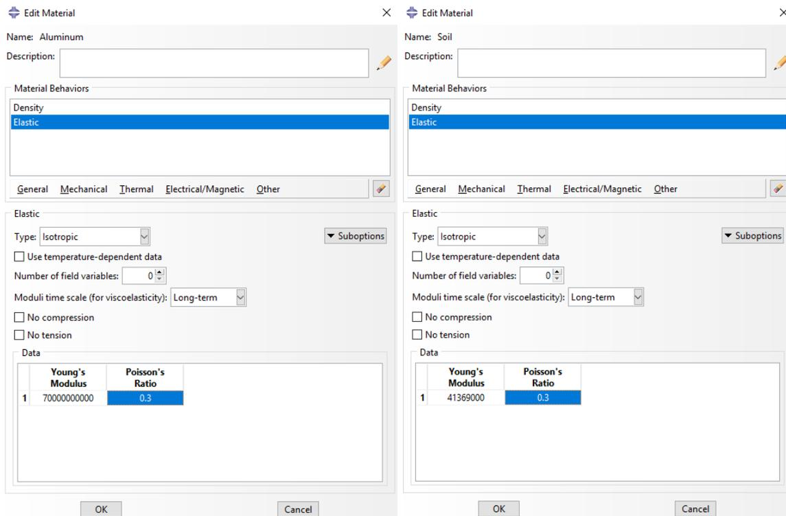
**Figure 2: Definition of the material properties in ABAQUS.**
