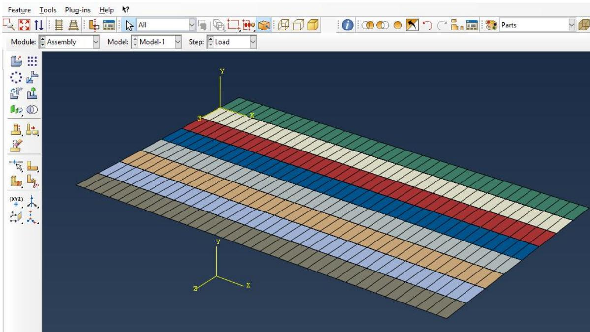
Figure 6: Panels assembly in ABAQUS.
