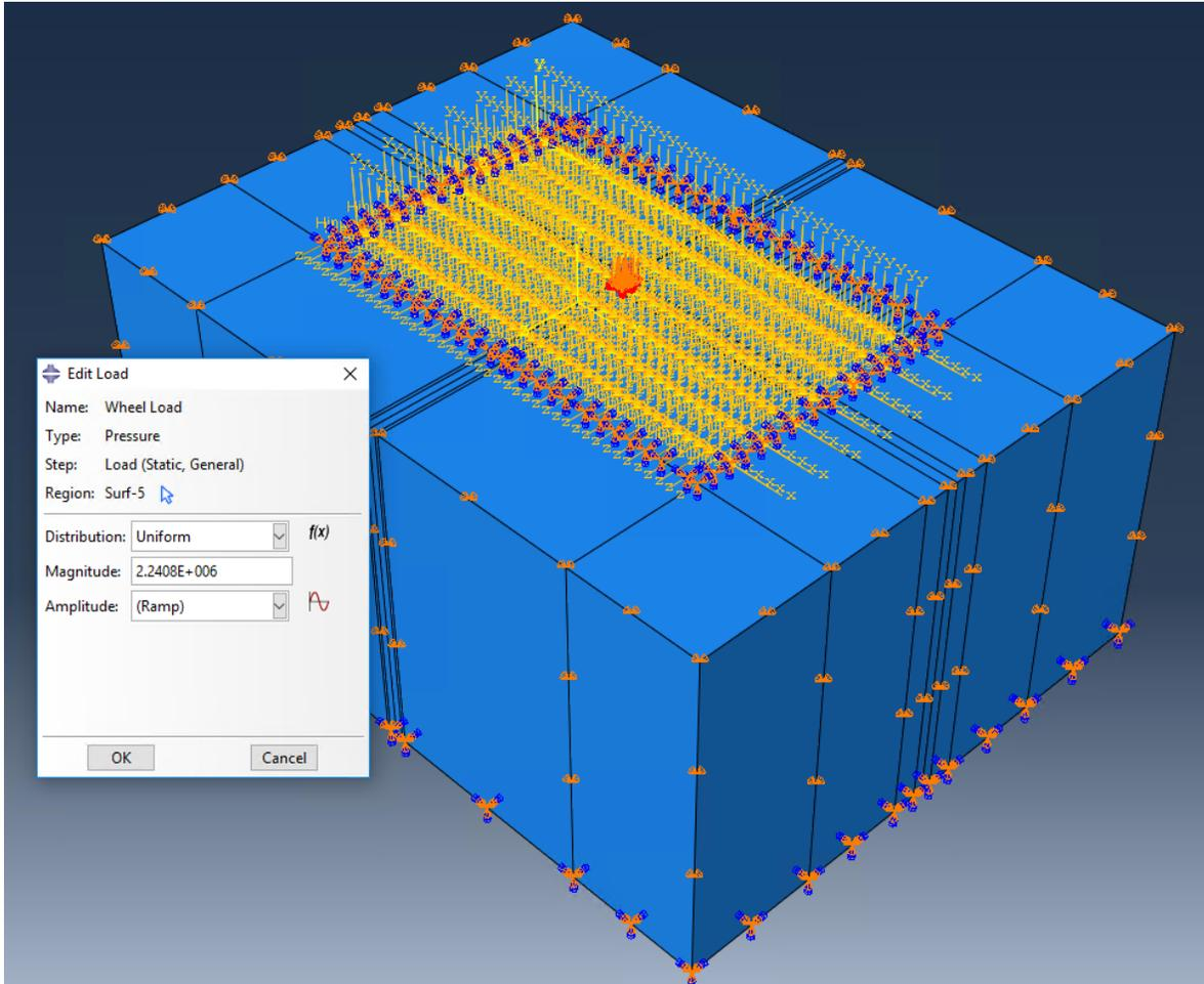
Figure 3: Definition of load pressure in ABAQUS.
