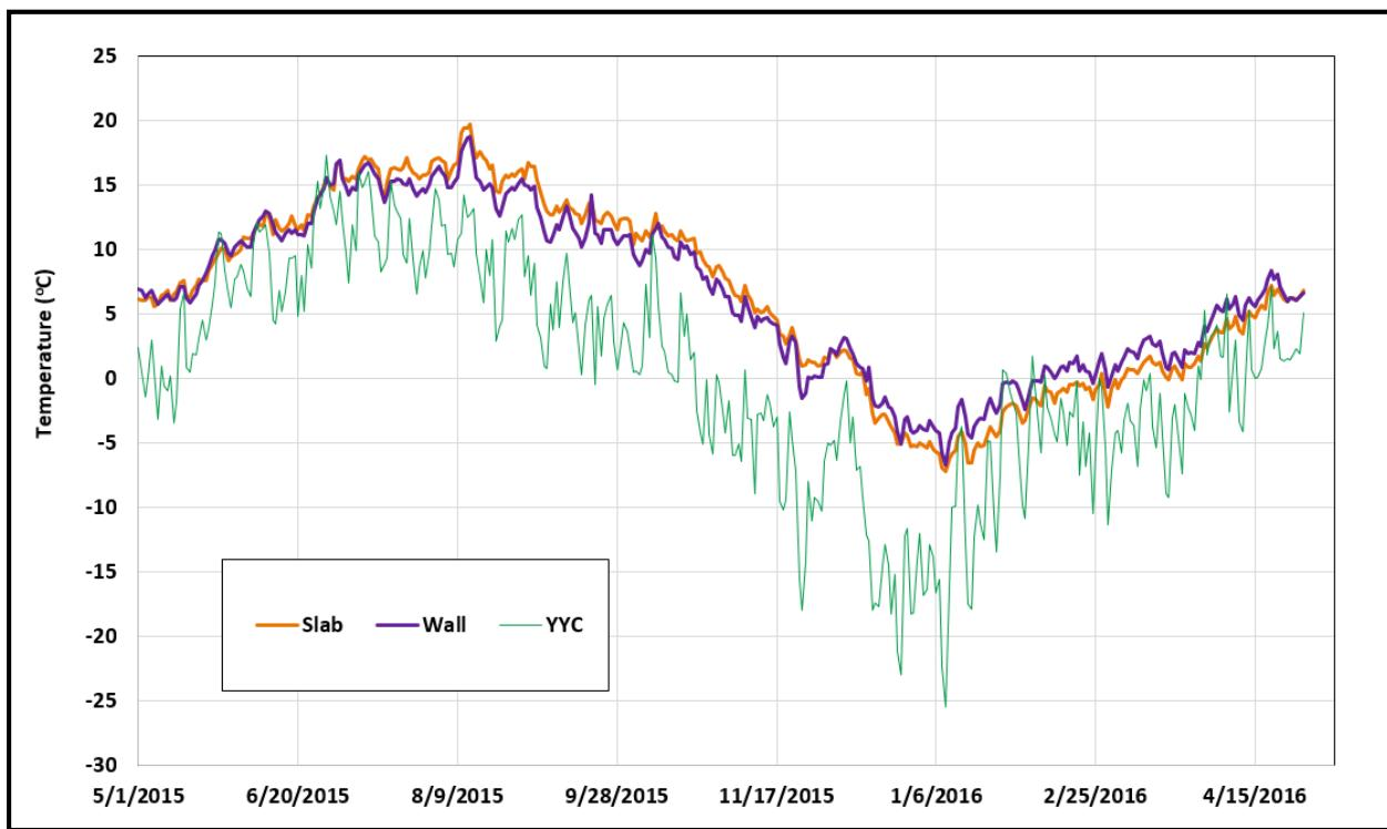
**Figure 12. Average of Minimum Temperatures for all Wall or Slab Sensors**
