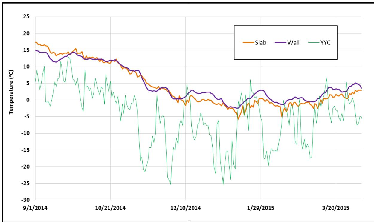
Figure 10. Average of Minimum Temperatures at Slab and External Wall, Dirt Side
