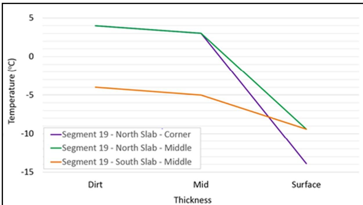
**Figure 16.** Temperature Distribution along Depth of Section for a Negative Temperature Differential
