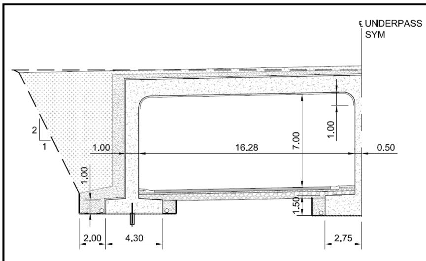
**Figure 2. Typical Tunnel Section**
