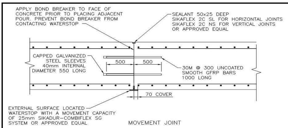
**Figure 3. Movement Joint Details**
