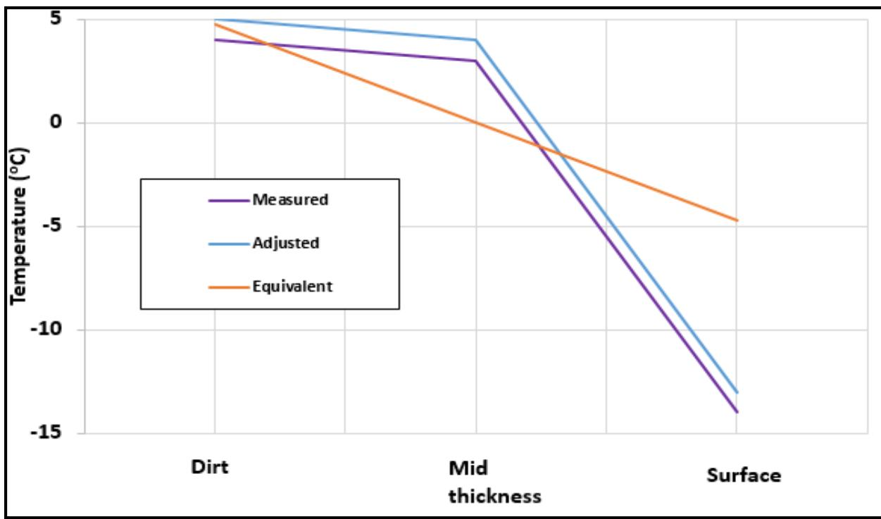
Figure 17. Calculated Equivalent Temperature Gradient
