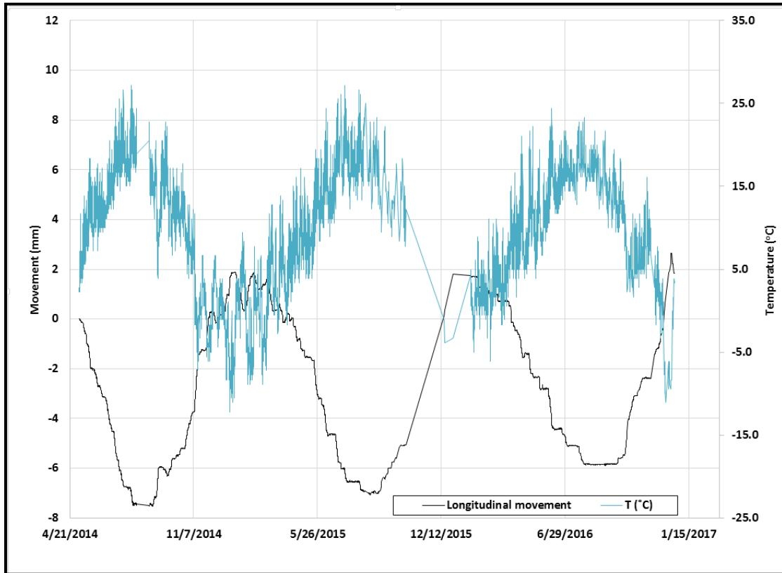
Figure 18. Longitudinal Movements
