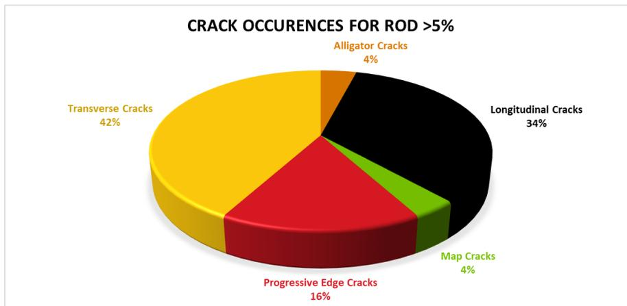
**Figure 9: Crack Type Distribution of Premature Cracking**
