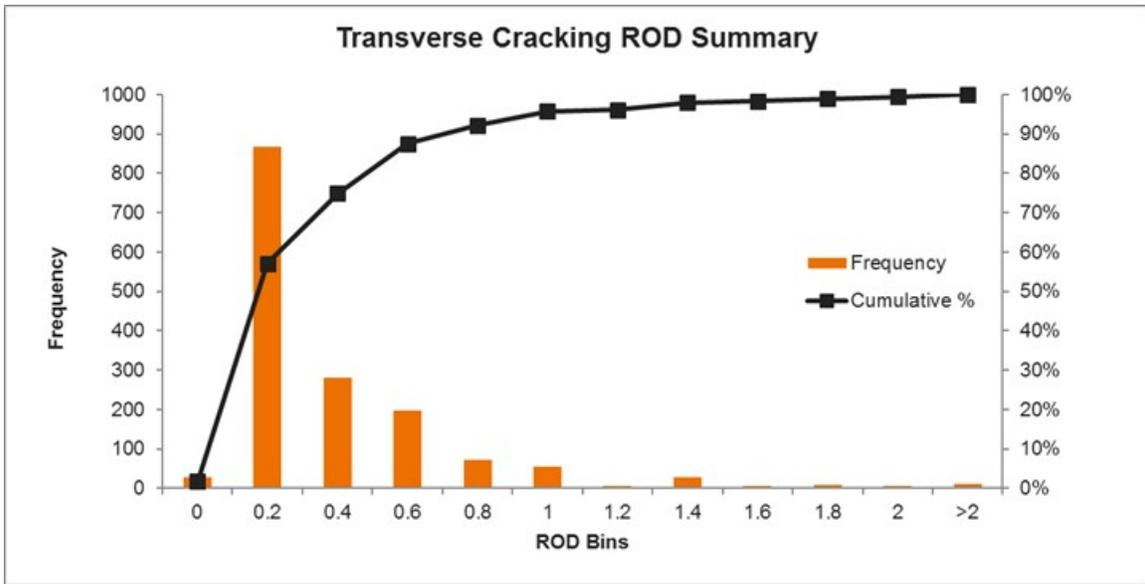
Figure 7: ROD Summary Transverse Cracking
