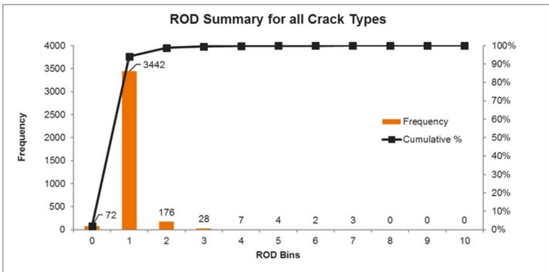
**Figure 2: ROD Distribution for all Crack Types**
