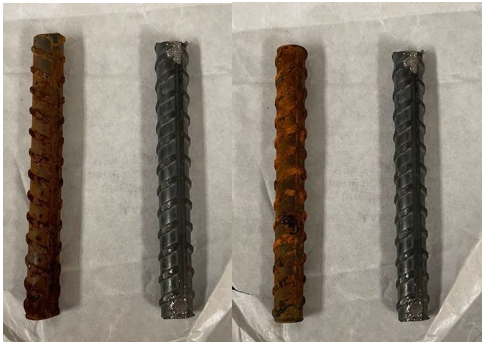
Figure 8: Samples G1 (Left) and H1 (right) in comparison to the control rebar sample.
