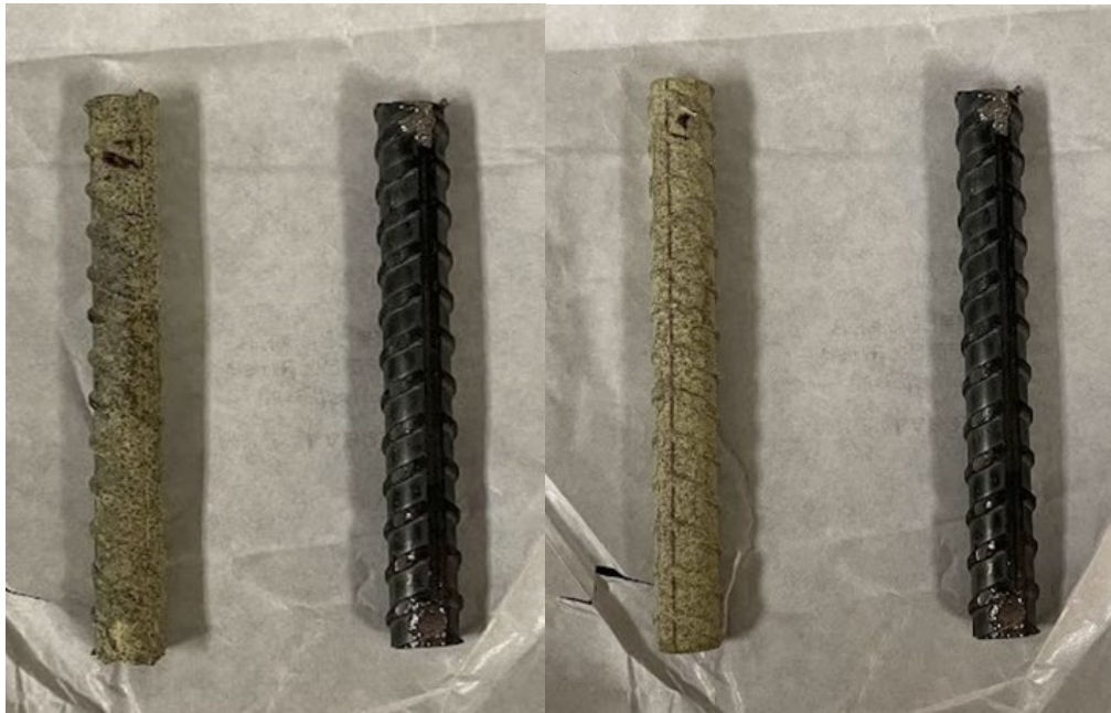
Figure 5: ECOST Samples A1(left) and B1 (right) in comparison to the control rebar sample.
