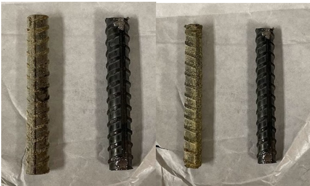
Figure 6: ECOST Samples C1(left) and D1 (right) in comparison to the control rebar sample.
