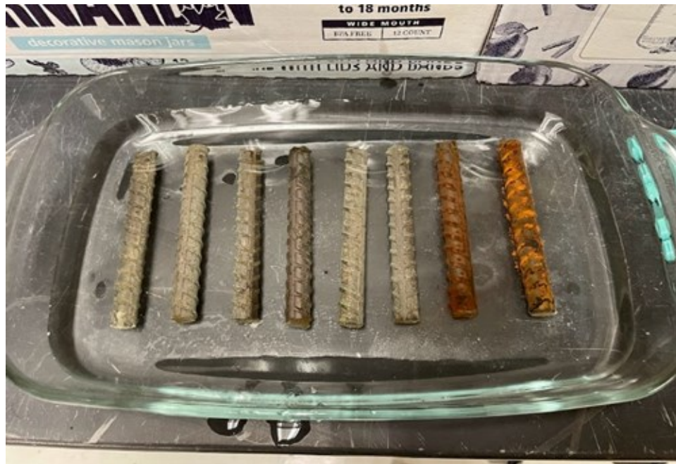
Figure 9: All samples from experiment 1 submerged in diammonium hydrogen citrate.
