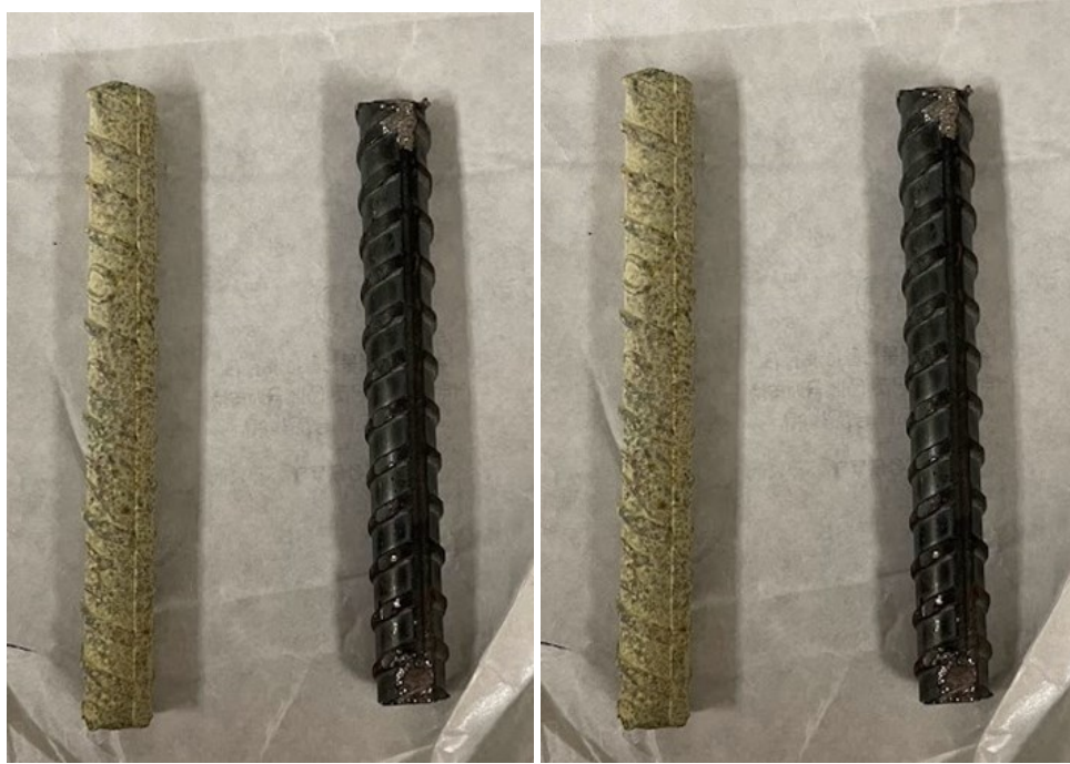
Figure 7: ECOST Samples E1(left) and F1 (right) in comparison to the control rebar sample.
