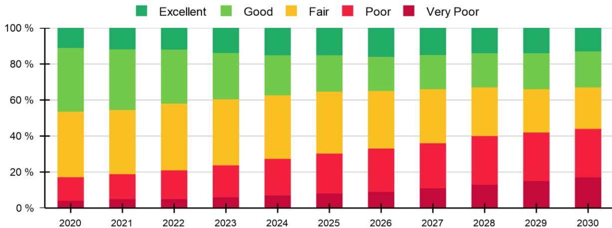
**Figure 7:** Network 10-year condition distribution using optimization
