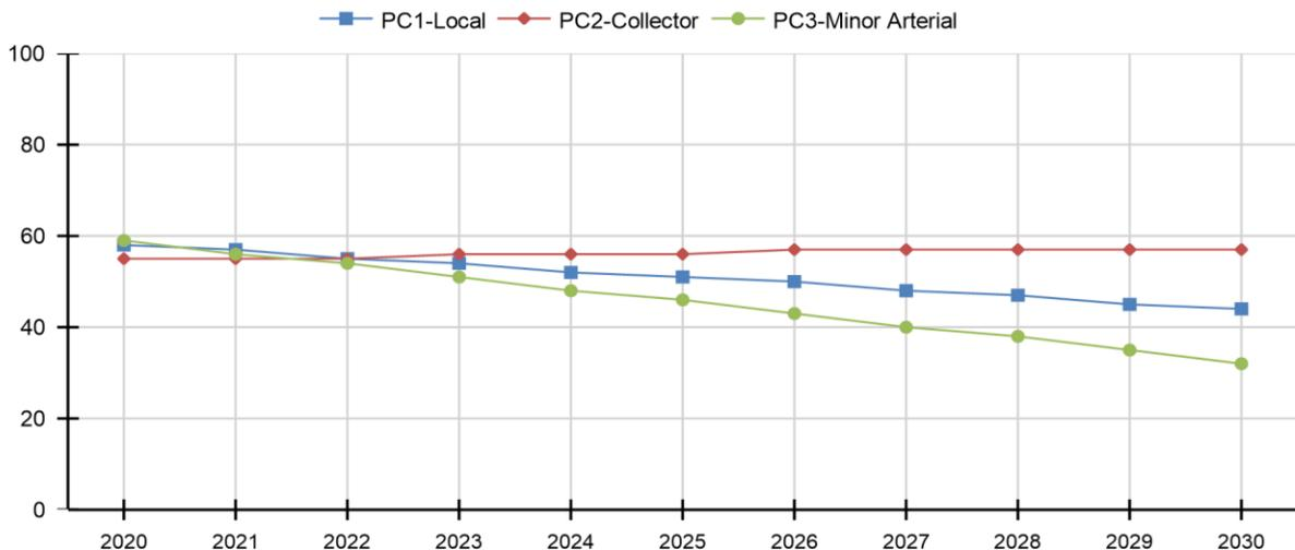
**Figure 4:** Condition projection based on functional class using prioritization
