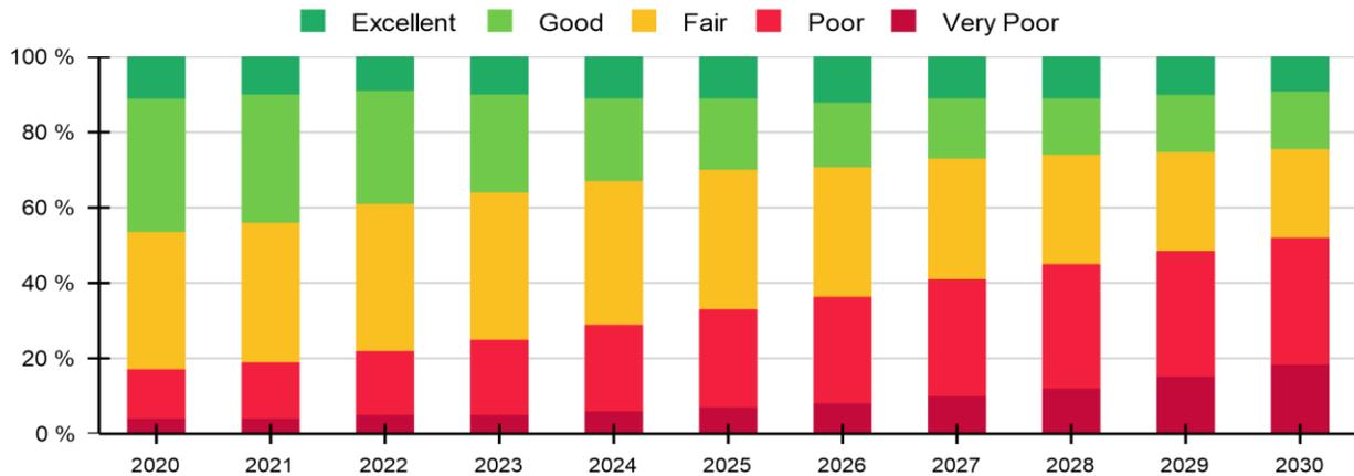
**Figure 5:** Network 10-year condition distribution using prioritization
