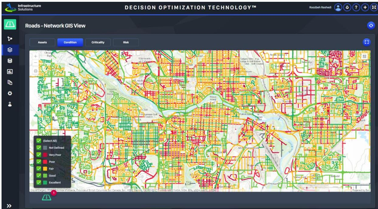
**Figure 3:** The City of Calgary's road network condition GIS view (DOT™ software)
