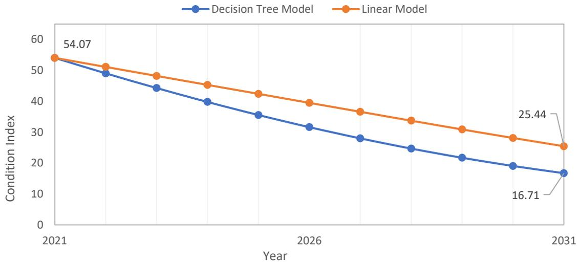
**Figure 10:** Do-Nothing deterioration projection for Collector roads
