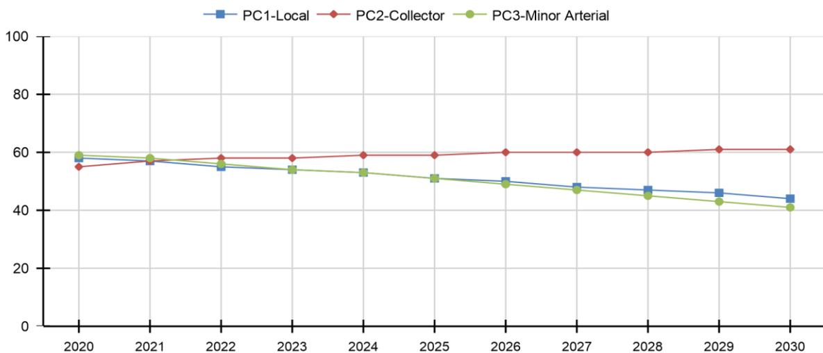
**Figure 6:** Condition projection based on functional class using optimization
