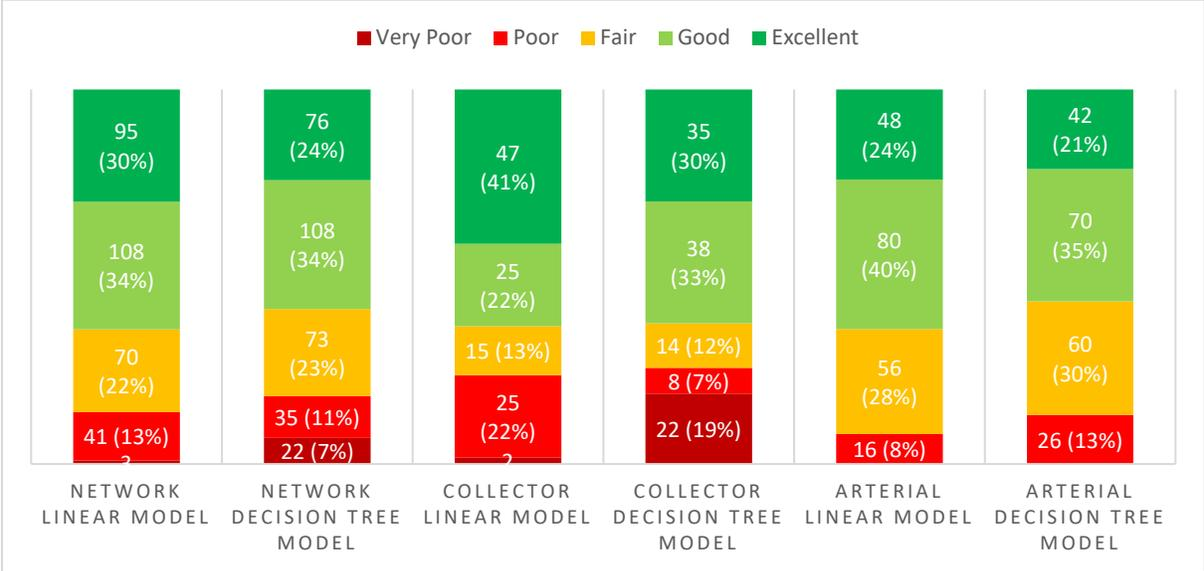
Figure 12: Kilometer of roads in different condition states by the end of the 10-year plan
