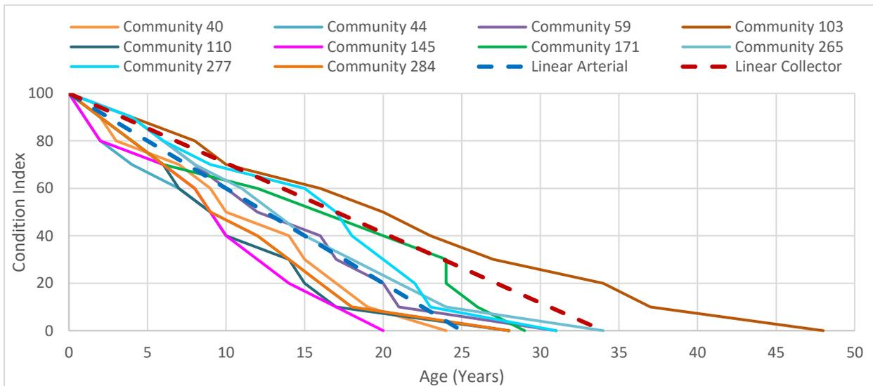
**Figure 9:** Decision tree and ESL-based deterioration curves
