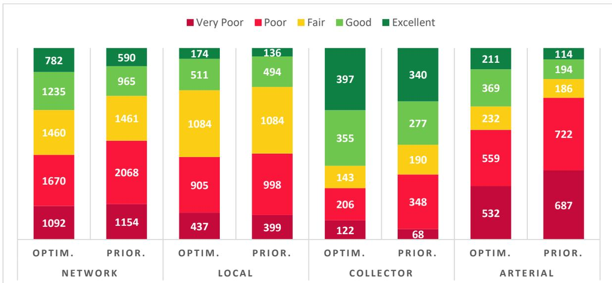
**Figure 8:** Kilometer of roads in different condition states by the end of plan (year 2030)
