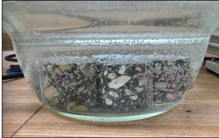
**Figure 3.** Vacuum saturation of AC Samples
