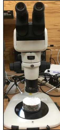
**Figure 8.** Stereomicroscope (SMZ1270i) with AC slice.
