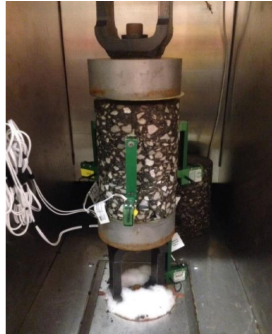
Figure 4: Typical dynamic modulus test setup
