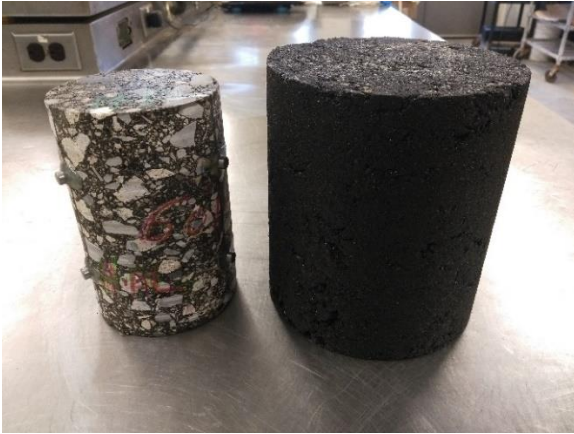
Figure 3: Gyratory compacted specimen before and after cutting and coring
