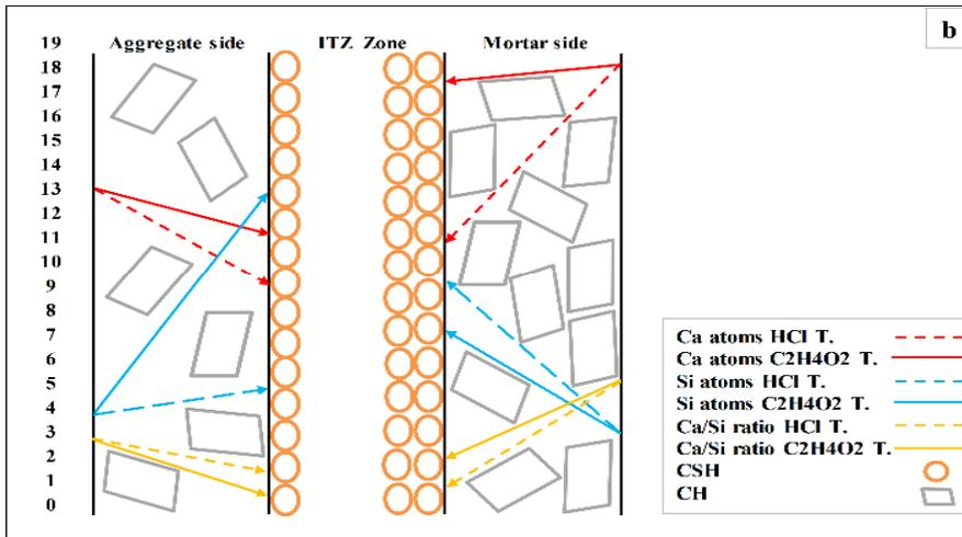
Figure 9: Schematic diagram of ITZ zone:- a: heat treatment at 250°C, b: acid treatments
