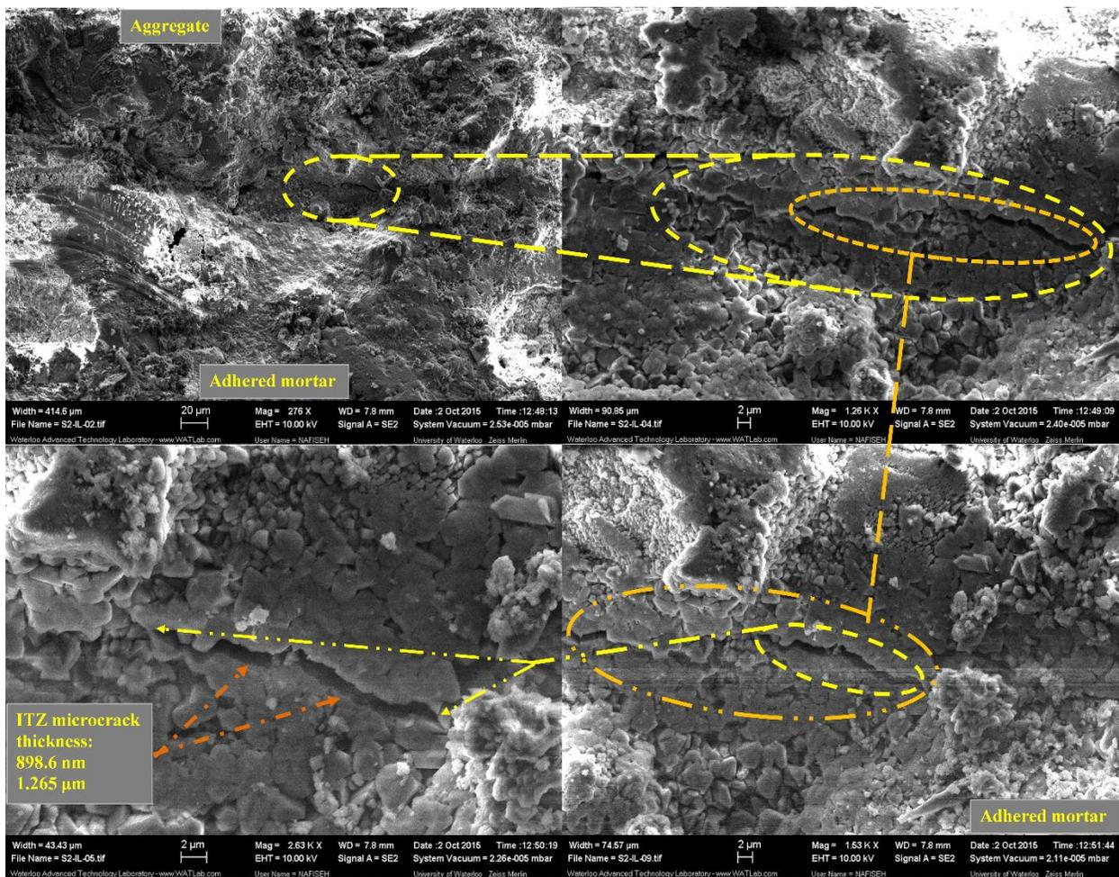
Figure 5: ITZ microcrack width to CRCA through heat treatment at 350°C
