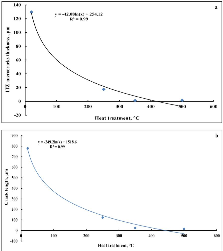
Figure 2: Behavior of ITZ microcrack through heat treatment:- a: width b: length
