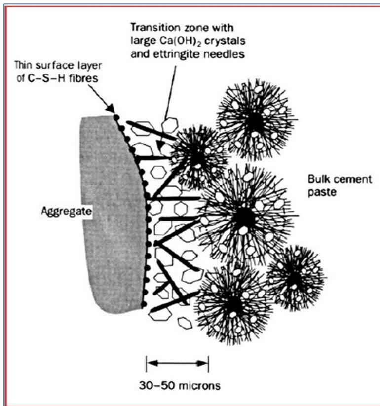
Figure 1: Schematic diagram of ITZ zone (Cement Chemical Composition and Hydration
