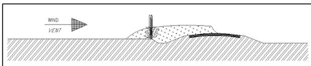
Figure 3 – Snow accumulation problem caused by fencerow obstruction
