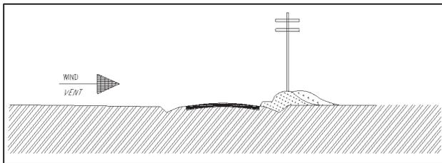
Figure 11 –Locate obstruction on downwind side of road
