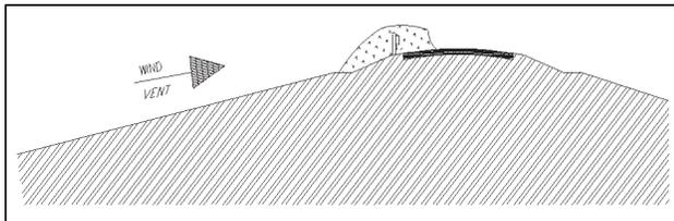
Figure 8 – Safety barrier causes snow accumulations along road
