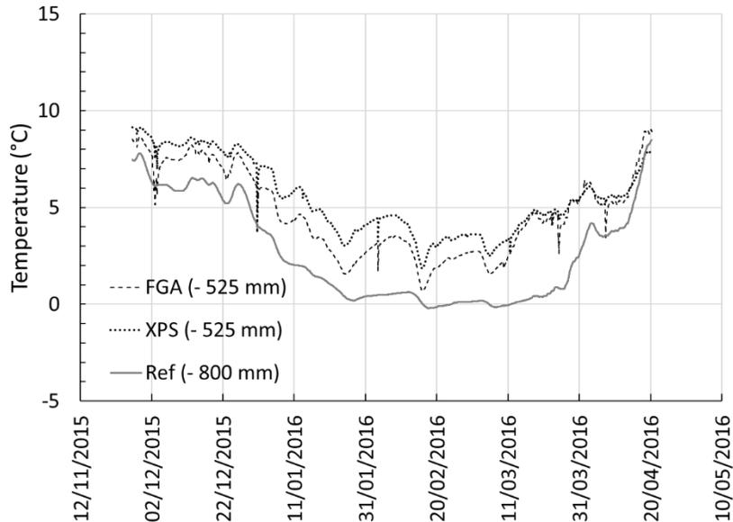
Figure 8 : Temperature under the insulating layers.
