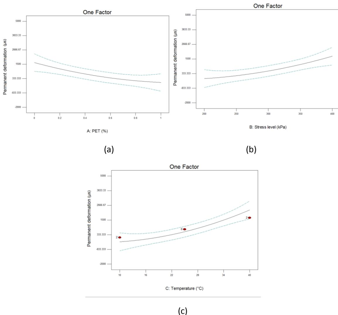
**Fig 3.** Effects of PET, stress and temperature variations on the permanent deformation property of PET modified mixtures
