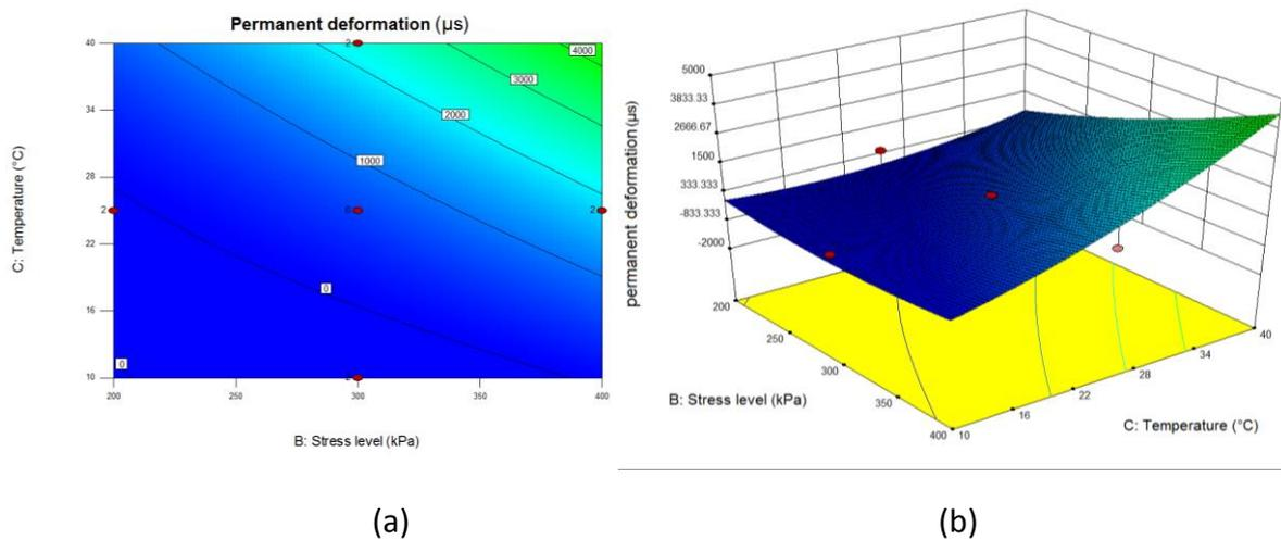
**Fig. 4.** Effects of stress level and temperature on the permanent deformation, 0.5% PET (2D and 3D)
