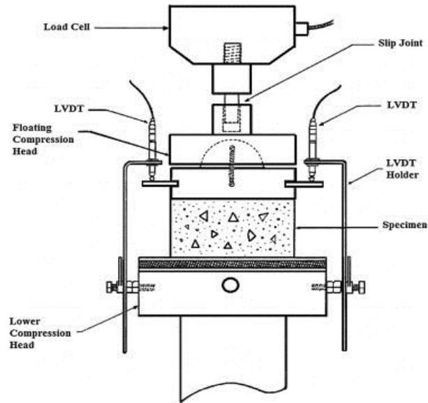
Fig. 1. Dynamic creep test set up [17]
