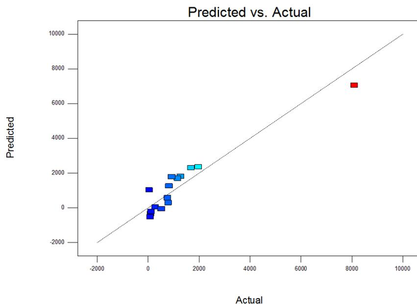
**Fig. 2.** Design-expert plot; predicted vs. actual values plot for permanent deformation responses
