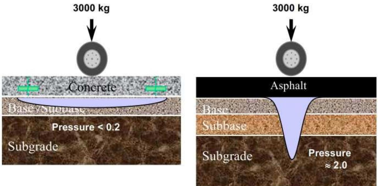
Based on the load distribution in PCCP, the volume of the excavation of the existing granular material was reduced to accommodate the concrete and the 200 mm designed thickness of the granular material. The remaining granular material from the ACP structure was intended to serve as the subgrade for the PCCP structure.
